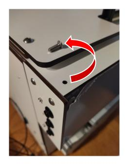
Using an Allen key for hexagonal screws, unscrew the screw on the top right of the button panel.
