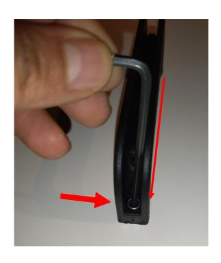
Use the Allen key to position the lock nut by sliding it along the key to position it in its housing.
