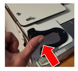
Reposition the barcode scanner holder (pack with the scanner).
