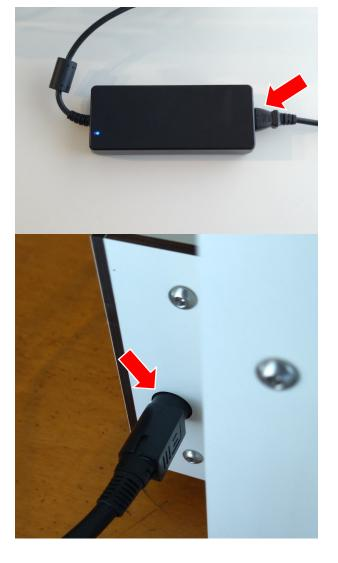
Connect a power cable to the 12V power supply.
